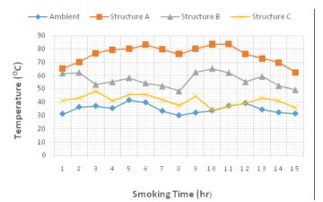
Figure 3. Temperature profile of the smoking structures at loading condition with 20 kg biofuel
