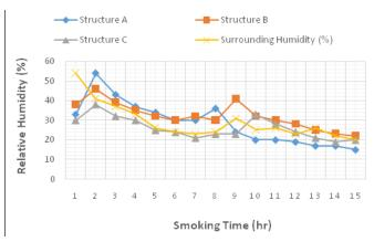
Figure 5. Humidity profile of the smoking structures
